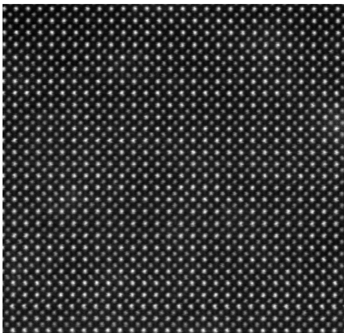
60kV HR-STEM image of highest-quality, ultra-thin lamella ( \langle 100 \rangle SrTiO 3 ) produced with Helios 5 UX DualBeam.
