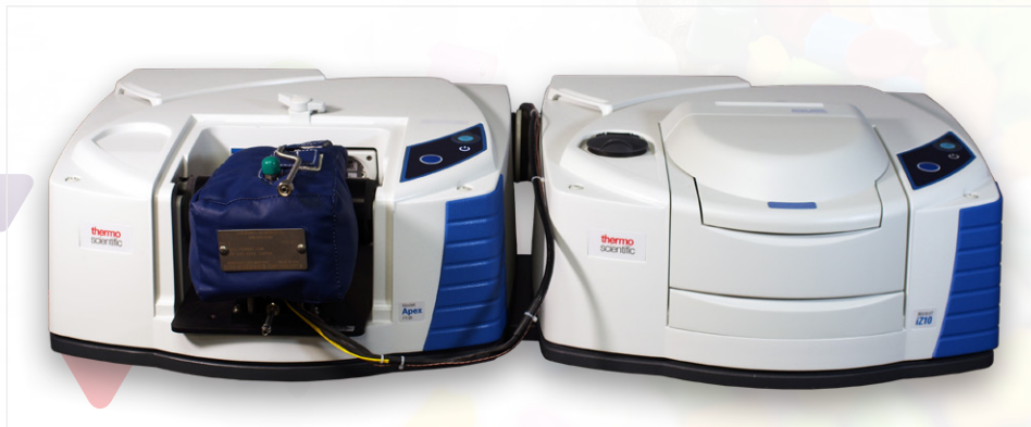
Multi-sample compartment multi-detector configuration for Nicolet Apex FTIR Spectrometer (left) with an iZ10 module (right). Main sample compartment configured with a jacketed 2 m gas cell and TE-MCT detector. The iZ10 module is configured with a smart OMNI transmission accessory.
