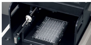
The Universal Platform Sampling accessory with Well-plate for the DXR3 SmartRaman Spectrometer
